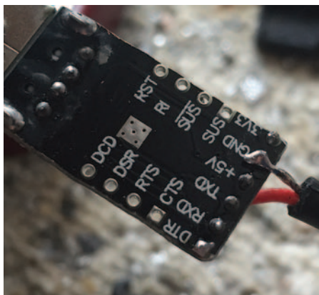
PHOTO 2: The RS-232 pin functions are clearly labelled. The red wire is connected to DTR (on the other side of the board).
