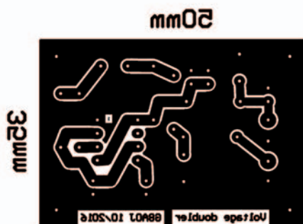
FIGURE 4: Reversed PCB foil pattern, 1:1 size. The dimension text should 'read right' on the foil pattern on the board.
