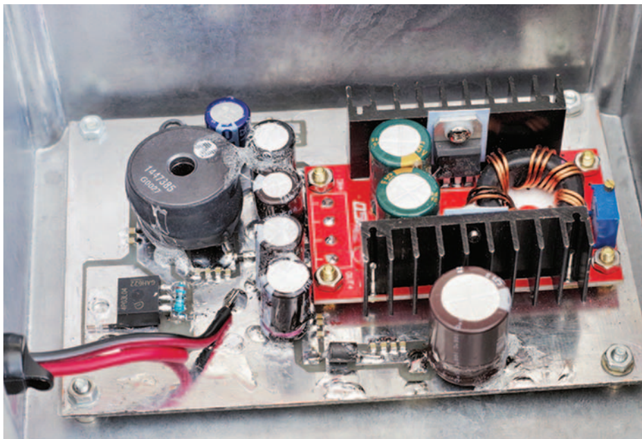
PHOTO 5: 12-28V SMPSU module with additional filtering components integrated onto a PCB. There is also a low power 12V output with extra filtering and P-channel MOSFET input polarity protection.
