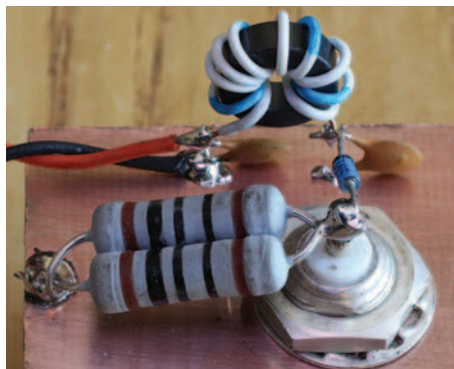
PHOTO 1: A simple 4W peak reading power meter that works from LF to VHF.
