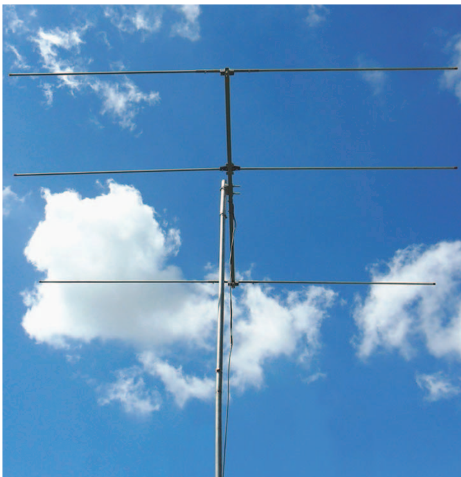
PHOTO 1: The 6m antenna built from the model's predictions
