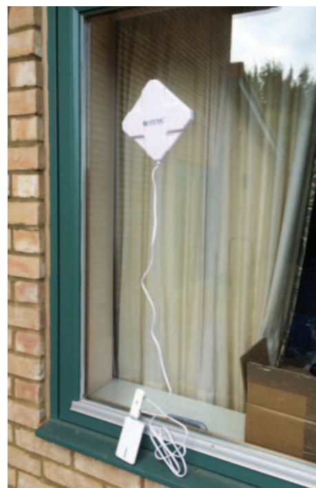
PHOTO 2: Wireless hotspot arrangement. Top to bottom: the eSYNiC antenna, connected to the Huawei 3G/4G dongle that is plugged into the TP Link portable Wi-Fi router.
